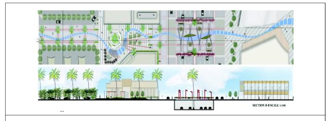
Figure 5: 3<sup>rd</sup> Street Crossing Prince Turki Street At Ground Level Where Vehicular Circulation is Separated Using an Underground Tunnel
