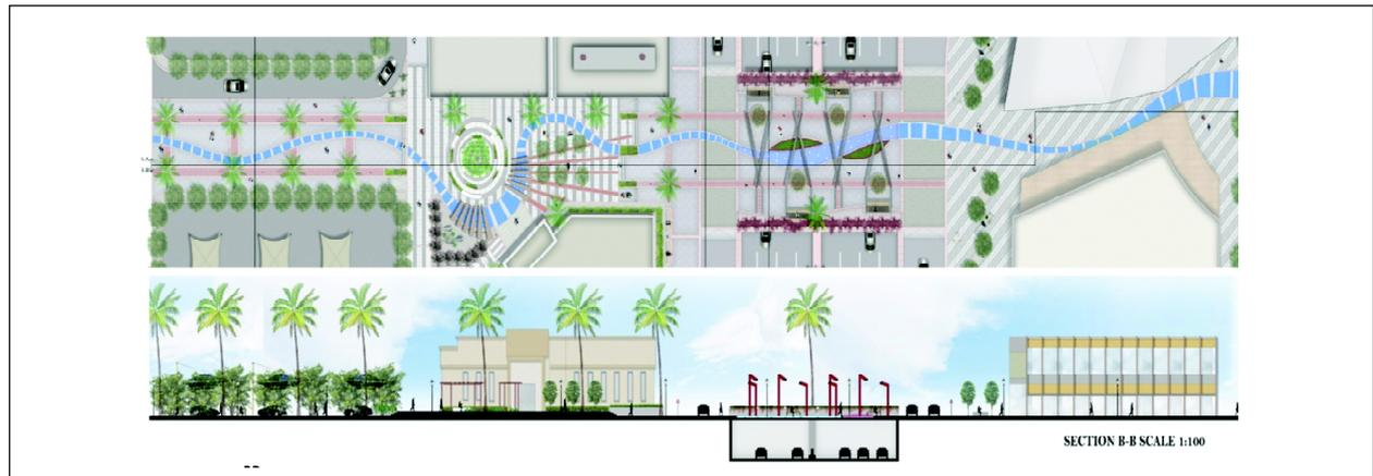
**Figure 5: 3<sup>rd</sup> Street Crossing Prince Turki Street At Ground Level Where Vehicular Circulation is Separated Using an Underground Tunnel**
