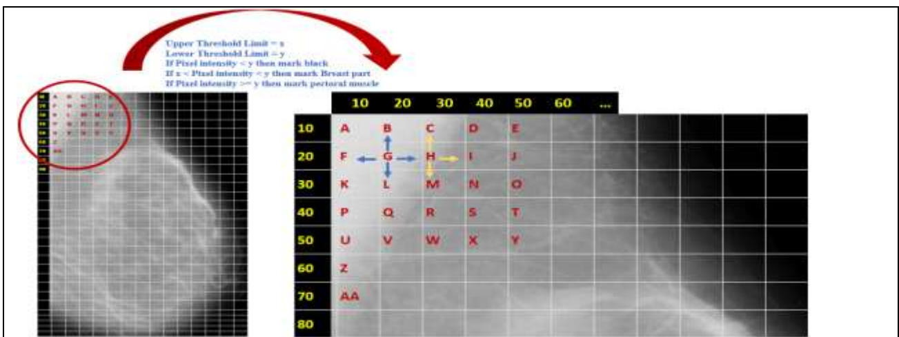
Fig. 5. Pectoral muscle detection using Breadth First Search Algorithm
