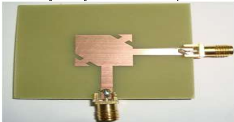
Photograph of Polarization-agile reconfigurable antenna when both strips are present.
