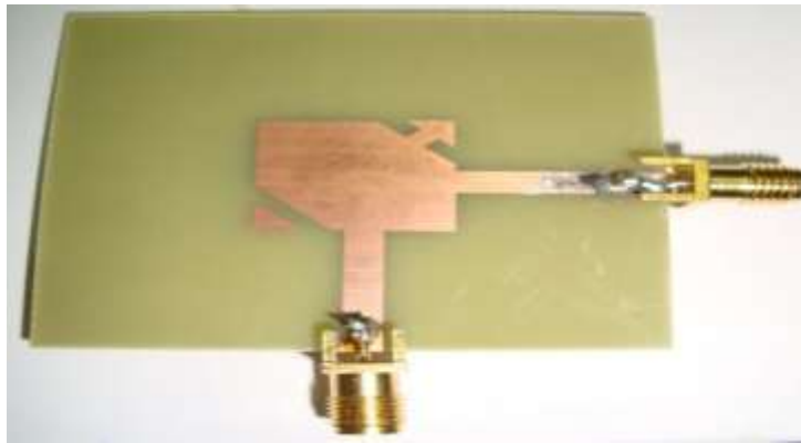
Photograph of Polarization-agile reconfigurable antenna when right strip is present. Photograph of Polarization-agile reconfigurable antenna when right strip is present.
