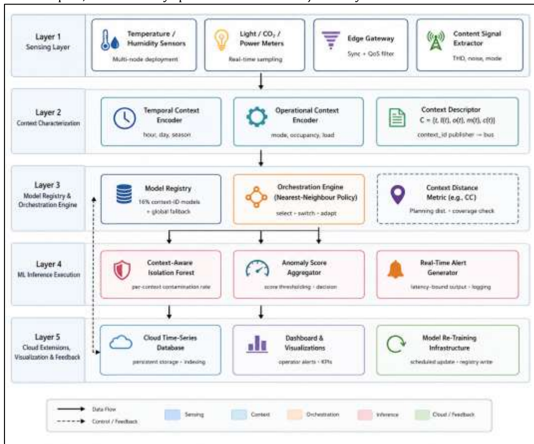
Fig. 1 Five-layer CASC-MO system architecture. The model orchestration engine (Layer 3) is fed by sensing and context extraction (Layers 1-2), which control context-specific inference (Layer 4). The cloud feedback loop (Layer 5) provides a way to schedule model retraining and registry updates
