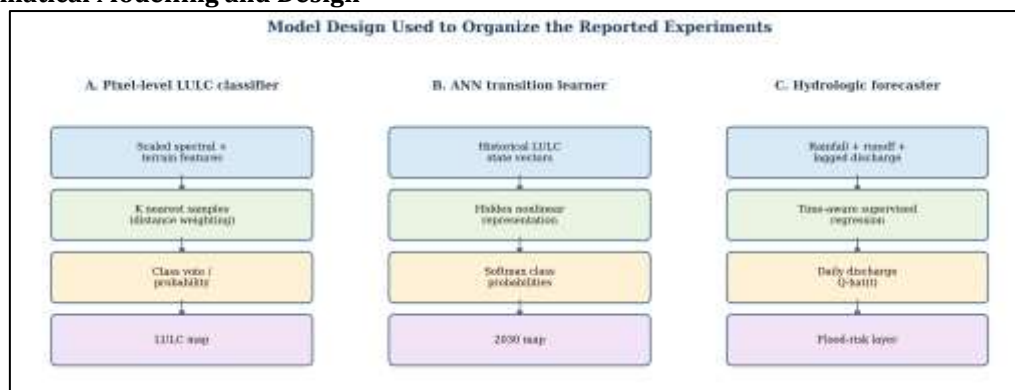
Fig. 2. Model design for LULC classification, ANN transition learning, and discharge forecasting.
