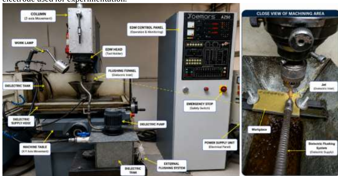
Figure 2: Experimental Setup of die-sinking Joemar AZ50 EDM with external Jet flushing system.
