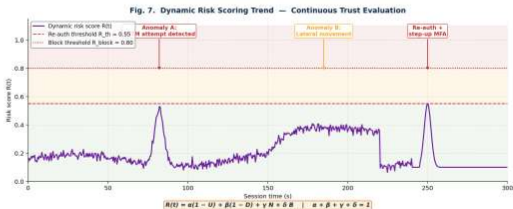
Fig. 7. Dynamic risk scoring trend during a 300-second session. Two anomalies are detected; the score crosses R_{th} , triggers step-up MFA, and recovers to baseline after re-authentication.
