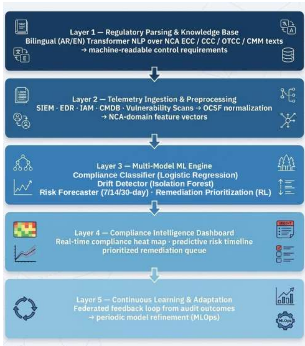
Figure 1. The proposed five-layer ML-based predictive and continuous GRC automation framework.
