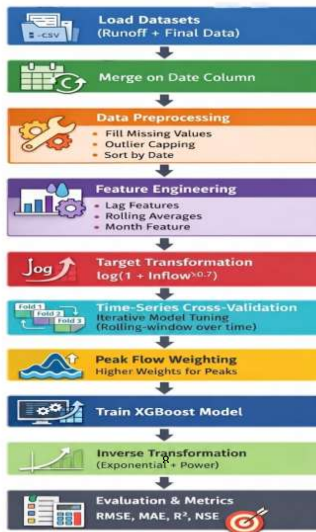
Fig. 3 Proposed Hybrid Feature Engineered XGBoost Framework For Reservoir Inflow Forecasting subsequent rainfall-runoff and inflow prediction modeling. The date attribute was converted into standard date time format and the dataset was arranged chronologically to preserve the temporal order required for
