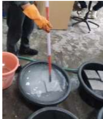
Fig 4.2: Acid solutions mixing
