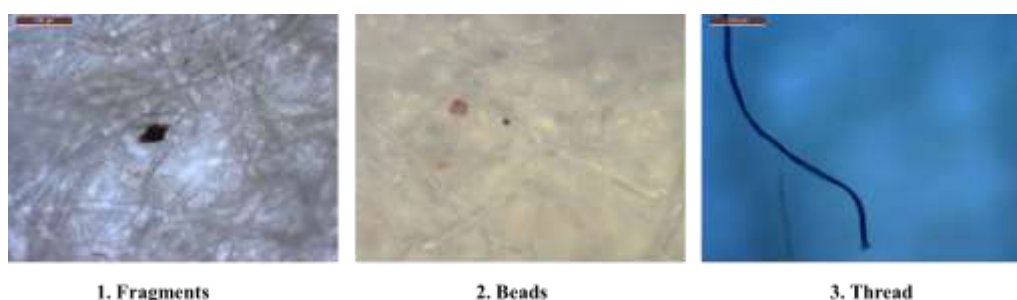
Figure 3. Example of original MPs images extracted from edible foods
