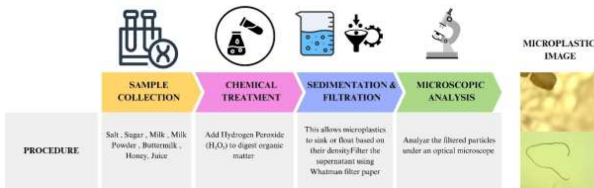
Figure 2 Scientific procedure for MP extraction from edible food
