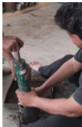
Fig. 5 – 7: Standard Proctor test.
