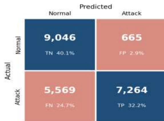
Figure 6. NSL-KDD test data confusion matrix for KNN intrusion detector.
