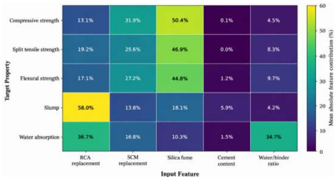
Figure 7. SHAP-based interpretation of the machine-learning predictions showing the global importance and direction of influence of major mixture variables for the concrete performance indicators.
