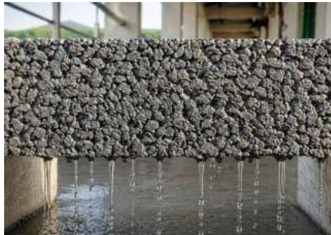
Figure 1: Visualization of water infiltration through the interconnected void structure of pervious concrete, illustrating permeability pathways and aggregate skeleton.
