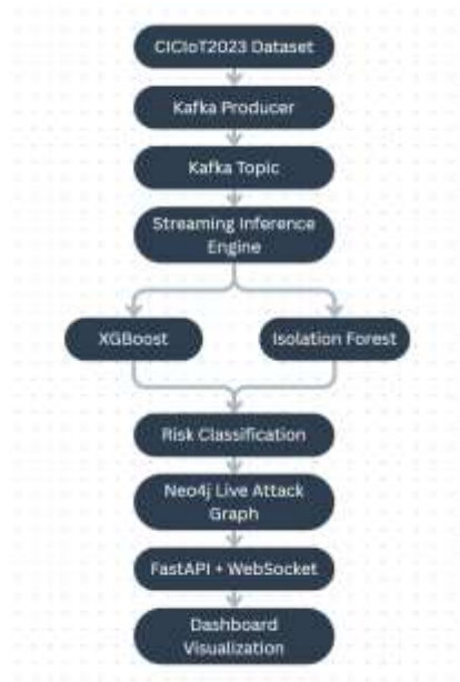
Fig. 1. ChainBreaker system architecture. Four layers share a single Neo4j instance; no secondary store exists.
