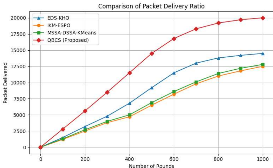
Figure 8. Comparison of the packet delivery ratio of the proposed algorithm with EDS-KHO, IKM-EPSo, and MSSA-DSSA-kmeans clustering techniques.
